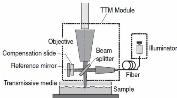
Fig. 4- Michelson type interferometric objective
