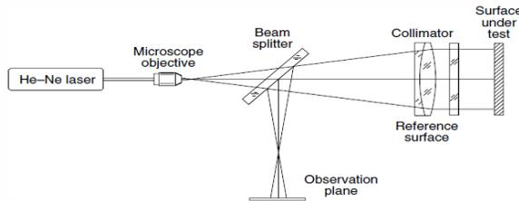
Fig. 2- Basic Fizeau interferometer configuration
