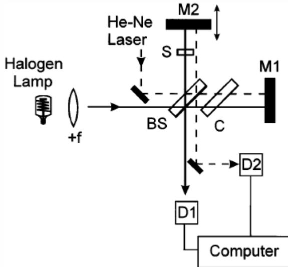
Fig. 5- Experimental setup for recording white-light interferogram.
