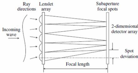
Fig 1. Schematic of a Hartmann-Shack sensor
