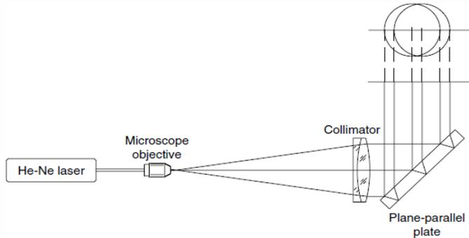
Fig. 3- Lateral shear interferometer
