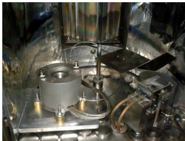
Figure 3: The technological room of the coating machine Leybold L560
