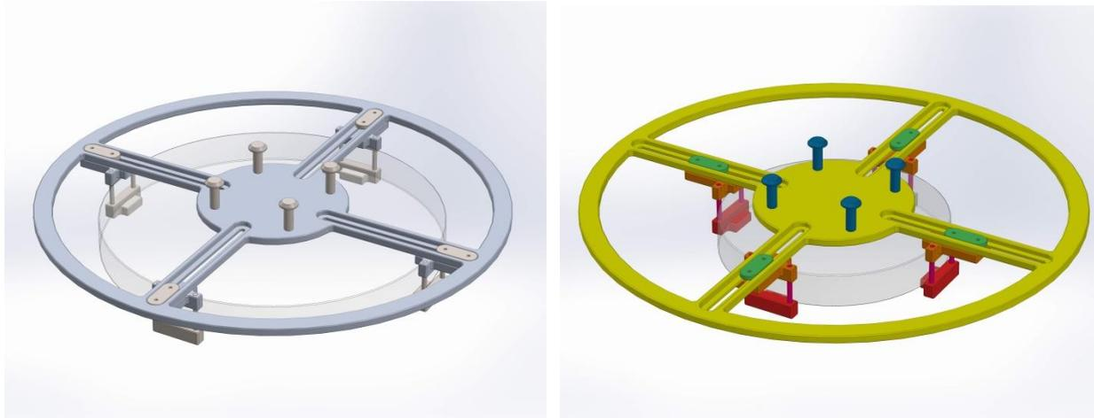
Figure 4: The holder device designed to sustain the large optical part during the coating
