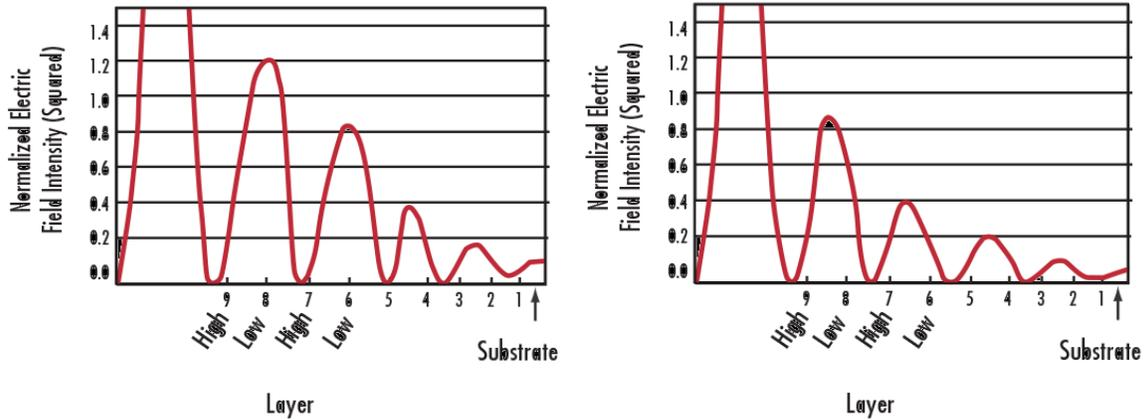
Fig. 1 Comparison of EFI to Layer within a Nine-Layer Stack Design with Layer Thicknesses Unoptimized (a) and optimized to decrease EFI (b) [1]
