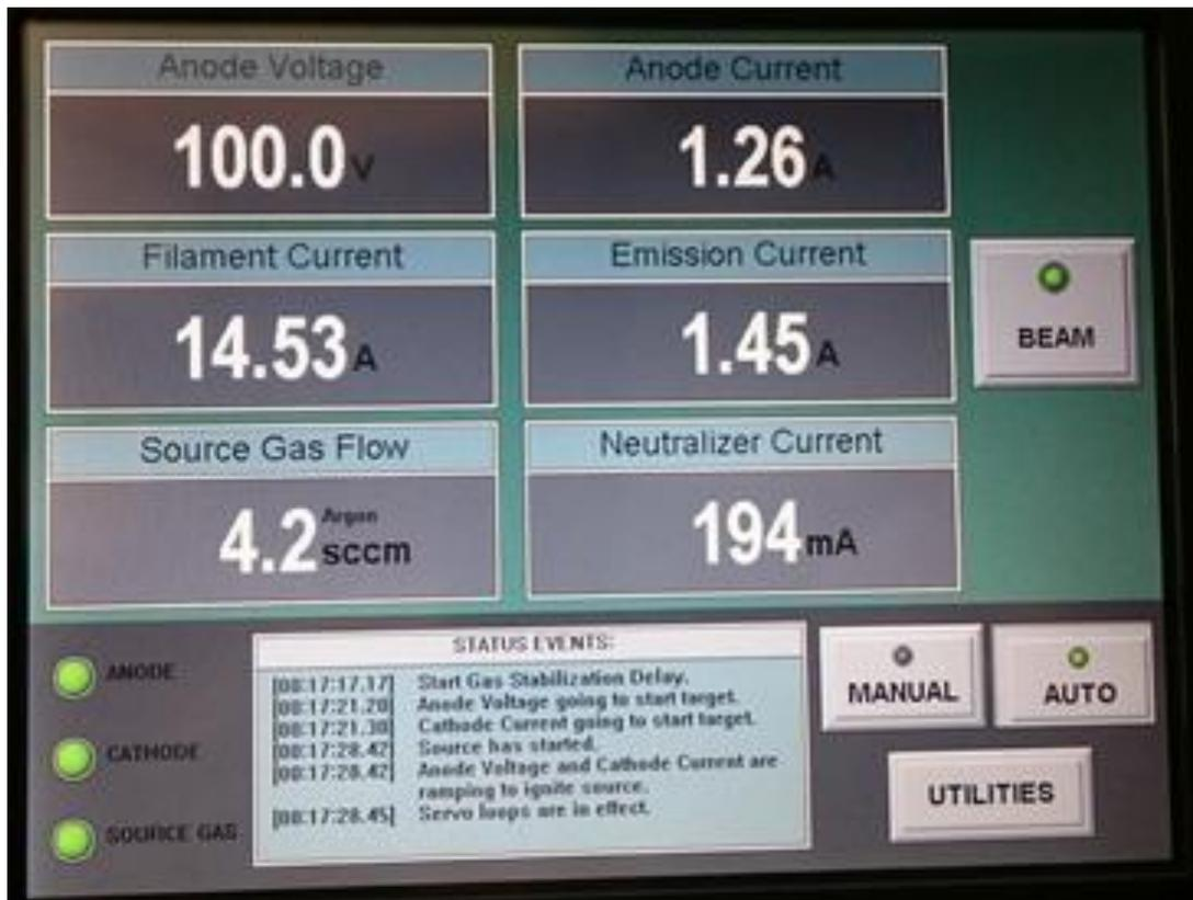
Fig. 4 - Screen capture with the parameters of the Ion Source
