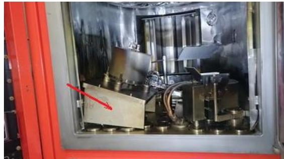
Fig. 2 - The tilted base of the Ion source
