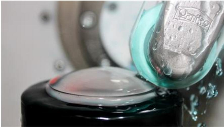
We will try to custom fit a spherical processing lathe with a special made and fitted device which will have an abrasive pad with a low grit size.
