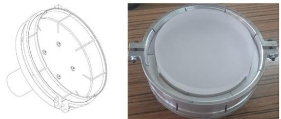
Fig.1 – The collet type chuck
