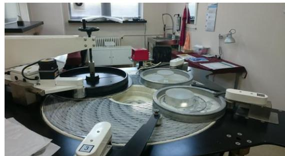
Fig.2 – The Lapmaster machine working to super-polish the mirrors substrates
