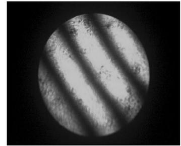
Fig.3 – Interferometric fringes of a measured optical surface
